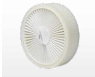
For insertion into wall sleeve. Suitable for ventilation systems from the iV-Smart+, iV14-Zero range. Note: Reduction of the AVF by approx. 15 %. (disposable filter, class F7 / ePM1 50 %, Ø 160 mm)
