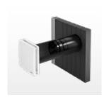
**iV-Smart+ Corner** (energy efficiency class: A+/A) consisting of: wall sleeve, Corner flat duct, reveal grille, inner cover with G4 filter, ceramic heat accumulator and inVENTron (Xenion reversible fan and guiding vanes). For wall thicknesses from 270 mm and at least 70 mm insulation.
