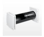
**iV-Smart+** (energy efficiency class: A+/A) consisting of: wall sleeve, weather protection hood, inner cover with G4 filter, ceramic heat accumulator and inVENTron (Xenion reversing fan and guiding vanes). For wall thicknesses from 270 mm.
