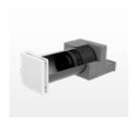
iV14-MaxAir Nordic (energy efficiency class: A+/A) consisting of: wall sleeve, Nordic external closure, outer grille, inner cover with G4 filter, ceramic heat accumulator and inVENTron (Xenion EFP reversible fan and guiding vanes). For wall thicknesses from 250 mm.
