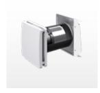
**iV-Compact** (energy efficiency class: A) consisting of: wall sleeve, special weather protection hood, inner cover with G4 filter, ceramic heat accumulator and inVENTron (Xenion reversible fan and guiding vanes). For particularly thin walls from a wall thickness of 140 mm.
