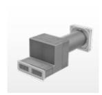
iV-Smart+ Nordic (energy efficiency class: A+/A) consisting of: wall sleeve, Nordic external closure, outer grille, inner cover with G4 filter, ceramic heat accumulator and inVENTron (Xenion reversible fan and guiding vanes). For wall thicknesses from 250 mm and at least 120 mm insulation.
