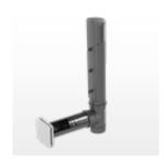
**iV-Smart+ Sylt** (energy efficiency class: A+/A) consisting of: wall sleeve, junction with condensate drain, weather protection hood, inner cover with G4 filter, ceramic heat accumulator and inVENTron (Xenion reversible fan and guiding vanes). For basements with wall thicknesses from 270 mm.
