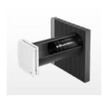
**iV14-Zero Corner** (energy efficiency class: A+/A) consisting of: wall sleeve with special sound insulation made from Inventin, Corner flat duct, reveal grille, inner cover with G4 filter, ceramic heat accumulator and inVENTron (Xenion reversible fan and guiding vanes). For wall thicknesses from 270 mm and at least 70 mm insulation.
