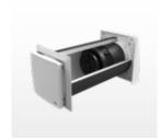
**iV-Office** (energy efficiency class: A+/A) consisting of: wall sleeve with special sound insulation made from Inventin, weather protection hood, inner cover with G4 filter, ceramic heat accumulator and inVENTron (Xenion EFP reversible fan and guiding vanes). For wall thicknesses from 260 mm.
