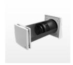
iV14-MaxAir (energy efficiency class: A+/A) consisting of: wall sleeve, weather protection hood, inner cover with G4 filter, ceramic heat accumulator and inVENTron (reversing fan Xenion EFP and guiding vanes). For wall thicknesses from 280 mm.
