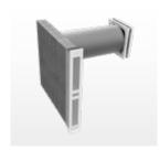
**iV-Twin+ Corner** (energy efficiency class: A+/A) consisting of: wall sleeve, Corner flat duct, reveal grille, inner cover, insert with two half-cylinder ceramic heat accumulators, two half-cylinder reversible fans and two G3 filters, vertical air volume flow separator. For wall thicknesses from 270 mm.
