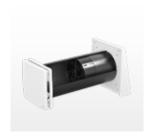
iV-Twin+ (energy efficiency class: A+/A) consisting of: wall sleeve, weather protection hood, inner cover, insert with two half-cylinder ceramic heat accumulators, two half-cylinder reversible fans and two G3 filters, vertical air volume flow separator. For wall thicknesses from 270 mm.
