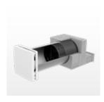
iV-Twin+ Nordic (energy efficiency class: A+/A) consisting of: wall sleeve, Nordic external closure, outer grille, inner cover, insert with two half-cylinder ceramic heat accumulators, two half-cylinder reversible fans and two G3 filters, vertical air volume flow separating element. For wall thicknesses from 270 mm.
