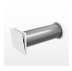
**iV-Light** (energy efficiency class: A+/A) consisting of: wall sleeve, round weather protection grille, extra-flat inner cover with G4 filter, ceramic heat accumulator and inVENTron (Xenion reversible fan and guiding vanes). For wall thicknesses from 290 mm.
