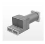
iV14-Zero Nordic (energy efficiency class: A+/A) consisting of: wall sleeve with special sound insulation made from Inventin, Nordic external closure, outer grille, inner cover with G4 filter, ceramic heat accumulator and inVENTron (Xenion reversible fan and guiding vanes). For wall thicknesses from 250 mm and at least 120 mm insulation.
