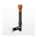
**iV-Smart+ Top** (energy efficiency class: A+/A) consisting of: wall sleeve, junction with evaporation pan, weather protection hood with insulation, inner cover with G4 filter, ceramic heat accumulator and inVENTron (Xenion reversible fan and guiding vanes). For installation directly under sloping ceilings (5-45°).
