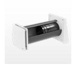
iV14-Zero (energy efficiency class: A+/A) consisting of: wall sleeve with special sound insulation made from Inventin, weather protection hood, inner cover with G4 filter, ceramic heat accumulator and inVENTron (Xenion reversible fan and guiding vanes). For wall thicknesses from 255 mm.
