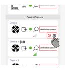
Press the "Radio signal weak" symbol of the component, that needs signal amplification (repeater necessary).
