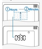
Initially the hour setting is flashing (1).
