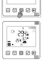
▶ Press the **mode key (a)** to confirm the paired components. (1)
